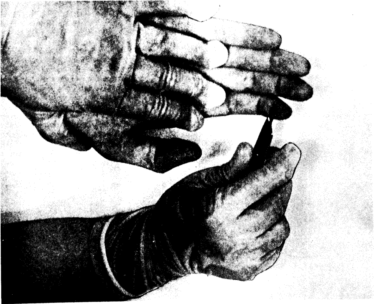
Figure G-30. Removing pattern area from first joint.
